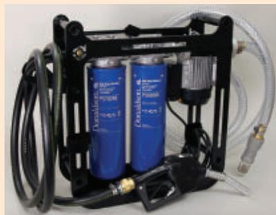
The Donaldson Fuel Cart is designed to remove contaminants from diesel fuel. The cart incorporates a Piusi Panther electric pump capable of 21 gpm to filter the fuel through separate particulate and water absorbing elements.
