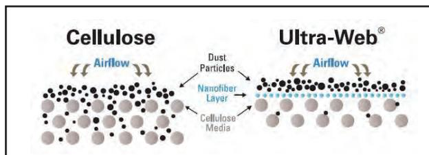
This illustration shows how Ultra-Web nanofibers allow more contaminant to be trapped on the surface of the filter media. This allows
