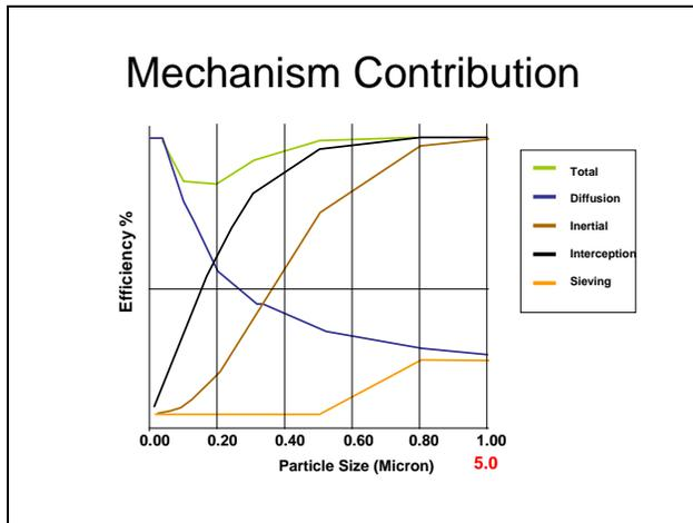
Figure 11. Contribution of Filtration Mechanisms in Air
