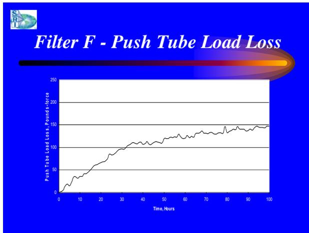
Figure 8. Shows Push Tube Pressure Loss in Pounds Force against Time in Hours<sup>5</sup>
