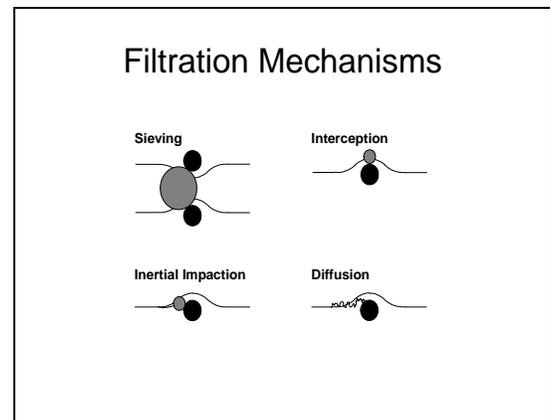
Figure 10. Filtration Mechanisms
