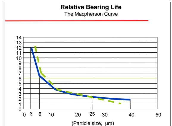
Figure 12. Macpherson Curve with Super-Imposed Line Depicted in Green Showing Estimated Size Distribution if Filters had been Tested Using NIST-Calibrated ISO Test Dust<sup>6</sup>
