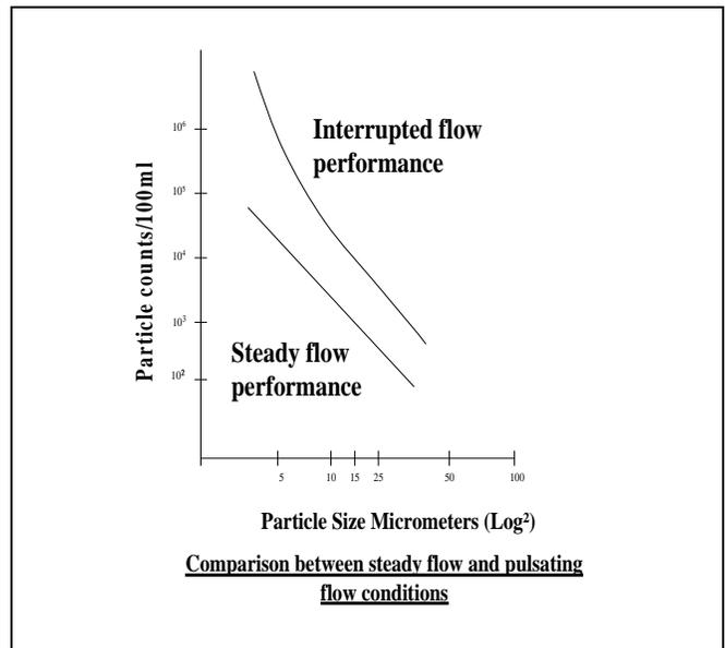
**Figure 6. Comparison of a Variation of Particle Size Retention of a Filter Media, Down Stream of the Media, when Subjected to Interrupted Flow<sup>2</sup>**
