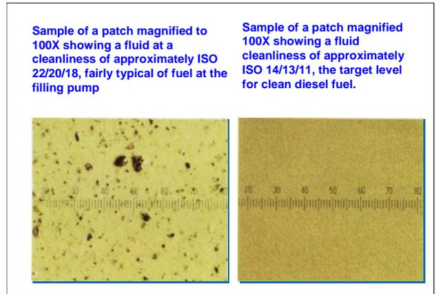
Figure 4. ISO 4406 Contamination Levels 22/21/18 and 14/13/11
