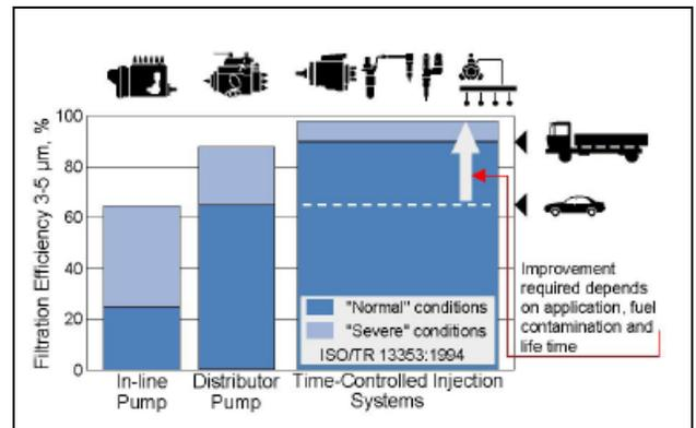
Figure 13. Projection of Fuel Filtration Requirements Based on Changing Injector Design by Robert Bosch GmbH<sup>4</sup>
