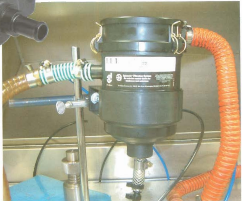
Donaldson Synteq XP CCV filter for off-highway application (in production) – test set-up for filter analysis
