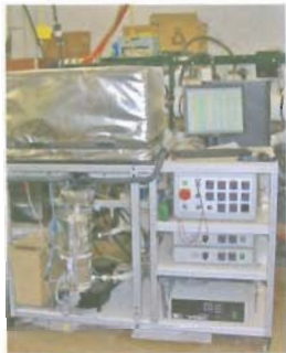
Oil mist generator and particle counter for CCV filter evaluation and development
