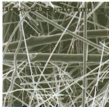
Donaldson Synteq XP media fibres: combination of synthetic and glass fibres and controlled dimensions and shapes
