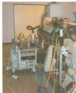
Engine blow-by analysis: particle size distribution measurement on engine dynamometer by Donaldson Leuven, Belgium
