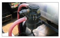
The Spiracle crankcase filtration system (CFS) eliminates harmful and unwanted crankcase emissions and allows the crankcase to be closed without degrading performance. It will reduce engine oil consumption (up to 6 gallons per year) and under hood odors/fumes.
