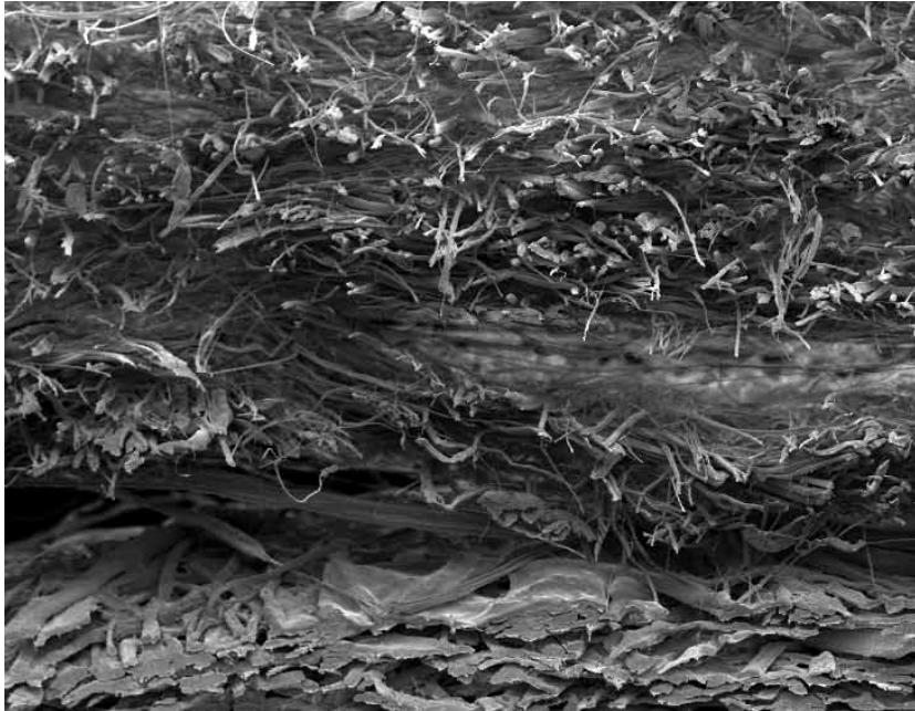
Donaldson Synteq™ fuel filter media shown at 100x magnification.
